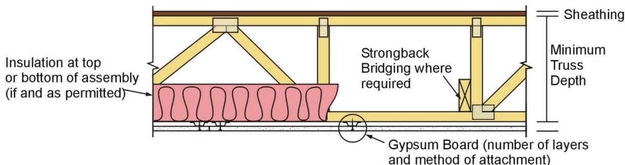
**Figure 1** – Generic fire rated wood truss assembly listing construction elements
